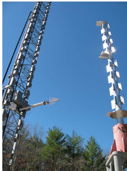
Outdoor 100' cylindrical near field range – Largest in the US.
